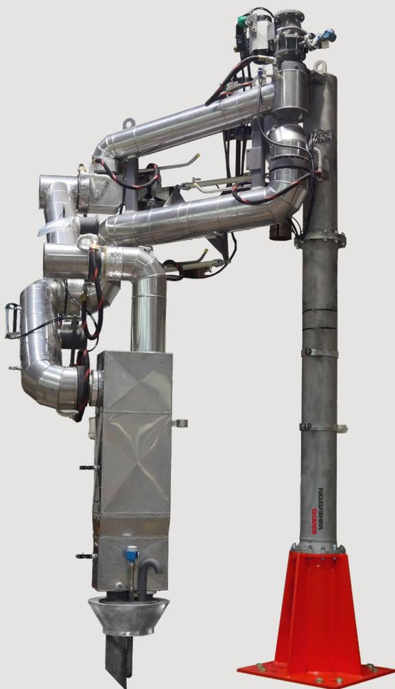
Parallel Loading arm with steam jacketed heating system and Picture
